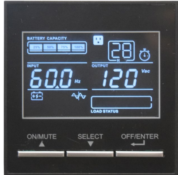
HMI showing key UPS parameters
