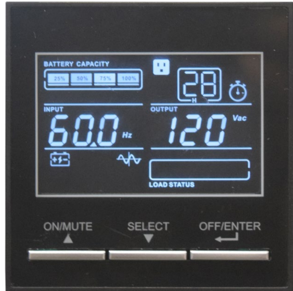
HMI showing key UPS parameters
